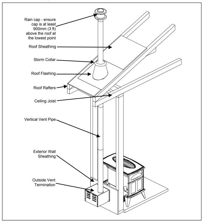
Figure 20: Exhaust Blower Installation; Vertical Termination.
